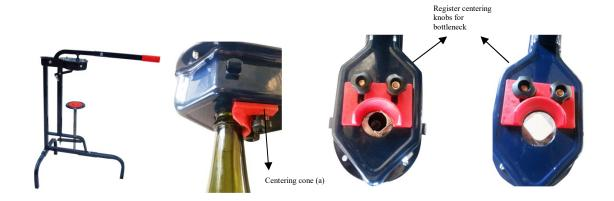
With adjustment of the level of insertion of the cap and centering cone (a) which allows the reduction of the inlet hole and ensures optimal alignment of the cap with the bottle. Ideal for natural champagne corks ø max 30.5 mm x h max 48 mm and bottles with a minimum height of 23 cm, maximum 34 cm. Preset for crown cap device ø 26 or 29 mm and bottles with a minimum height of 17 cm, maximum 28 cm.
